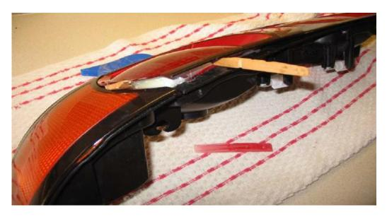
Before working in the peg (refer next picture), prise the tab on the amber lens free of the tail light backing body. It needs to lift a little to be able to free the lip of the amber over the red lens.
