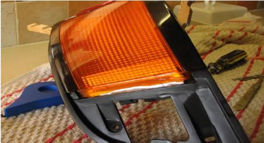
You may need to put the unit back in the oven at this stage for a few minutes to be able to lift the amber enough to free it from the channel in which its sits as the channel is deeper than you think.
