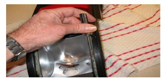
With the casing nice and warm, you can use White Spirit and a clean cloth to wipe away mastic that's got on the edge of the casing, and also bend the edge of the backing in case it needs a slight re-profiling to regain its original shape after having the pegs wedged in it.
