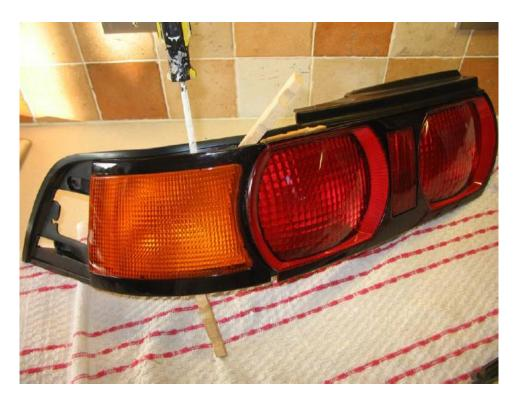
At this stage, you should be able to work the edge of the amber lens out of the recess next to where the amber (or red) triangle section sits.
