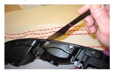
After prying the lens up a little from the unit, then insert a couple of halves of wooden clothes pegs. Wooden pegs being softer reduce the risk of damage to the lens or unit casing than when using metal instruments such as screwdrivers or similar.
